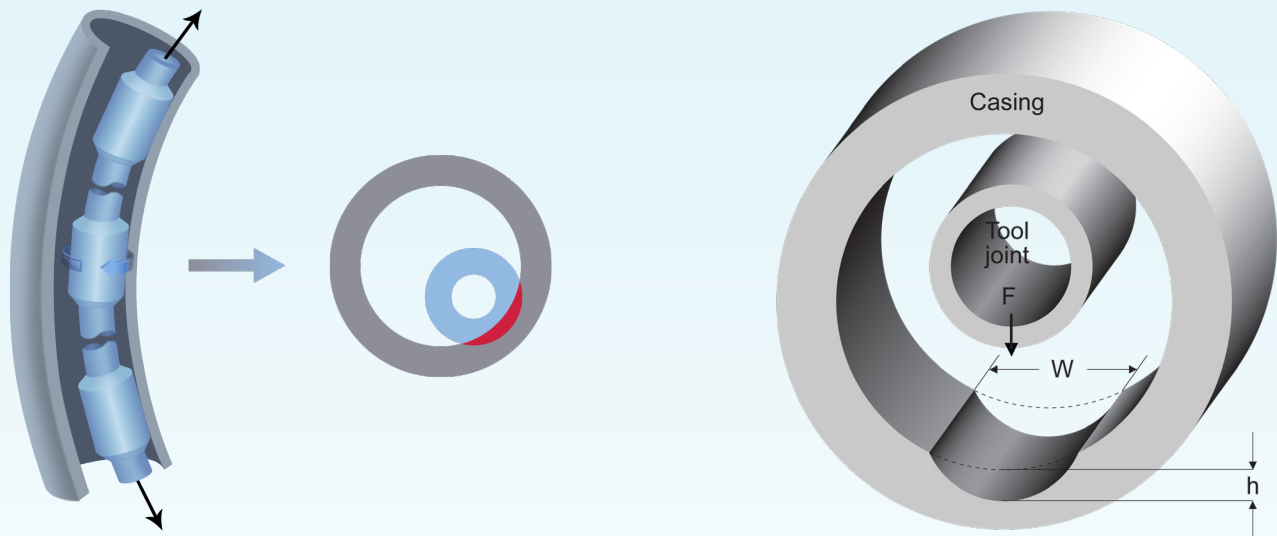
Figure 2. Rotating Tool Joint Wears Crescent Grooves in Casing
