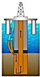
Reverse - pump down CK lines - Multiple lines
