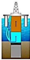
Pump down CKB lines to clean up riser - Multiple lines
